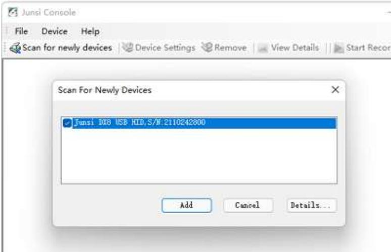
1. Connect DX8 with PC via USB port (make sure USB driver has been installed), and run the software, then the system will find new equipment, so just click “Add”
