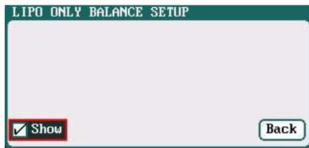
➤ *Balance Only* is the program only to equalize the individual cells through balance port to reduce the voltage difference.
