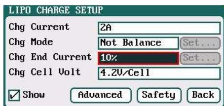
➤ The charger first charges with constant current (CC) according to the user setting, then turns to constant voltage (CV) when the charging voltage reaches the peak point. In the CV phase the current gradually falls, and the charger will terminate charging when the current falls below the percentage of the configured charge current.
