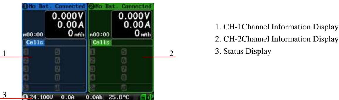
➤ When the selected input power supply does not support recovery discharge, the icon "1" in the lower left corner is gray; It is displayed in green when recovery discharge is supported.
