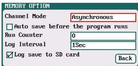
Channel Mode: *Asynchronous (default); Synchronous*
