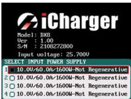
➤ There are different parameter setting of these four types of power supply, the user can set in **SYSTEM MENU** → **Input Limit** see details on "**Input Limit Setup**".
