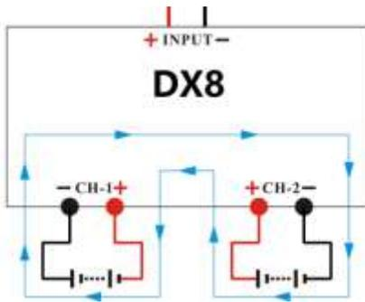
1. In any channel of the charger, *MEMORY SETUP* → *Discharge* → *Regenerative Mode* → *To channel*, to select Charging battery; then connect the battery for discharging to this channel, and start the discharge program, and this channel will be in discharging stand by status;
