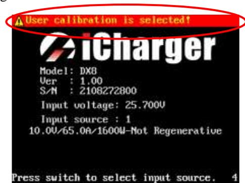
➤ If the user selects *User Calibration*, the corresponding message will appear in the interface after booting the charger, as shown in the up picture above.
