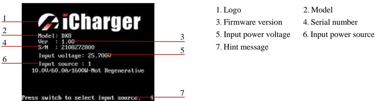
System will delay **5 seconds** after booting, during this period, long press **<●>** button to change the input source type, while pressing any other buttons to enter the initial interface.
