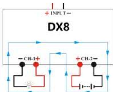
1. Connect the resistance or bulbs to any channel of the charger;
