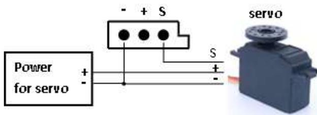
Select *SYSTEM MEN*→*SERVO TEST* to enter servo test interface; insert Servo into multi-function port to test.
