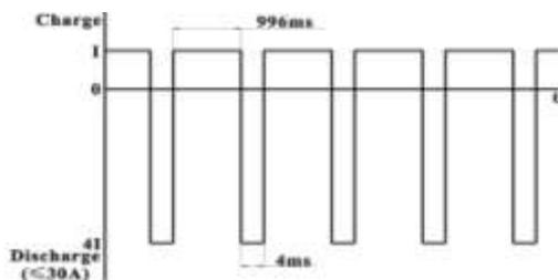
Reflex charge mode only supports NiMH and Pb battery. It does not support lithium battery. Using reflex charge mode to charge battery can reduce effectively the heating of the battery. Go to the MEMORY SETUP → Charge → Chg Mode to select Reflex mode.
