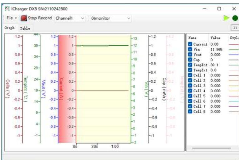
3. Start the charge/discharge program of DX8, then detailed data and curves can be viewed
