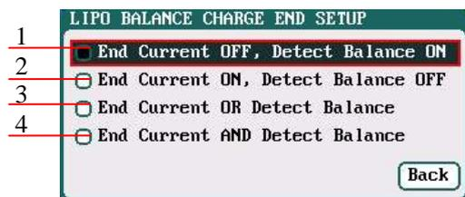
1. The charger will stop balance charge if detects the Balance condition is met, and the End Current condition is invalid
