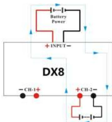
which is when the power supply for the charger acts as "battery power", the charger will regenerative charge for "battery power" during the process to discharge the battery. Go to MEMORYSETUP → Discharge → Regenerative Mode → To input.
