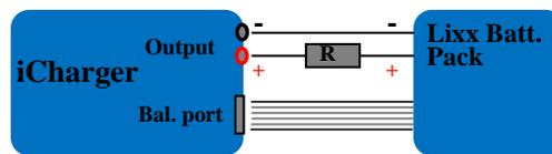
In this mode, the lithium battery discharges through the iCharger and R,  $P = P_i + P_r$ , ( $P_i$  is the charger’s wasted power capacity;  $P_r$  is wasted power capacity by resistance).  $P_i$  is limited by the set charger’s maximum discharge power capacity.
