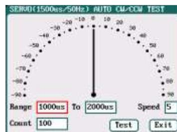
**Liner Test:** When turning the knob, the pointer deflects with the setting value of *Step*, and the servo responds accordingly.
