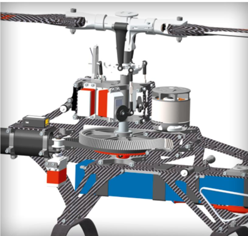
\*CRS (Chronos-Rotorhead-System) High precision rotor head geometry
