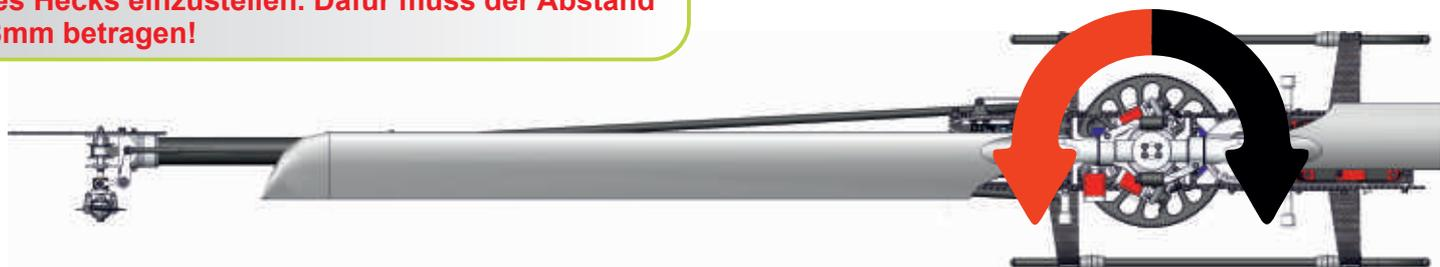
Tail Rotor compensation: Observe helicopter from top while rotating the entire machine clockwise as viewed from top (red arrow). The slider must move away from the tail case (black arrow). When helicopter is rotated counter-clockwise (black arrow) slider should move toward the tail case (red arrow).
