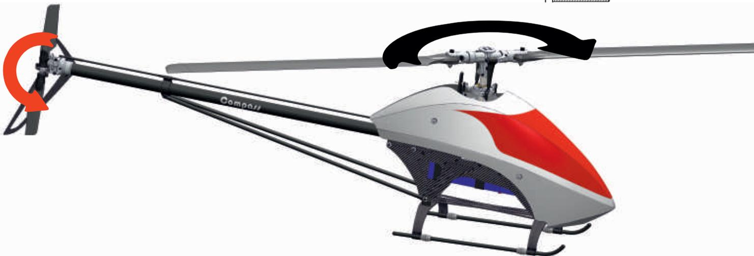
When main rotor rotates clockwise (black arrow) tail blades should rotate counter clockwise (red arrow) as observed from right side of the helicopter. If not, the belt is twisted in the incorrect direction (see step 47). Be sure that main rotor and tail rotor blades are installed in the correct direction.
