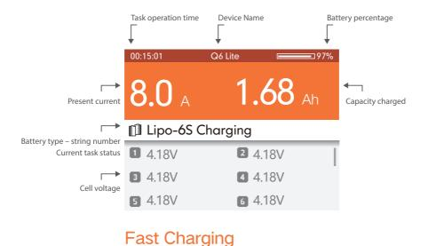
Rotating the shuttle key during operation can switch the displayed information in the lower half of the screen, which are cell voltage, cell internal resistance and working parameter. The cell voltage and internal resistance can only be displayed in the mode of balance charging (3 minutes).
