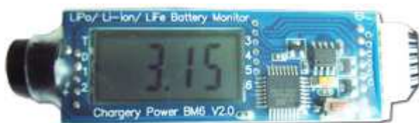
lowest cell voltage setup for alarm
